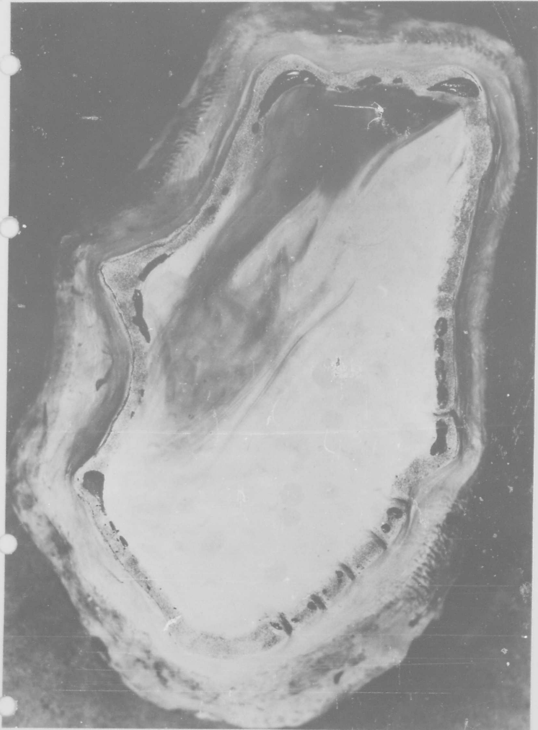
FIGURE 5 - MODEL OF BIKINI SHOWING WATER MOVEMENT WITH SOUTHEAST WIND, A FEW SECONDS BEFORE THE PHOTOGRAPH WAS TAKEN, A DROP OF DYE WAS PLACED AT THE TARGET CENTER; THE SURFACE CURRENT CARRIED SOME DYE TO THE NORTHWEST; THE REMAINDER WAS CARRIED SOUTHEAST ALONG THE REEF.
